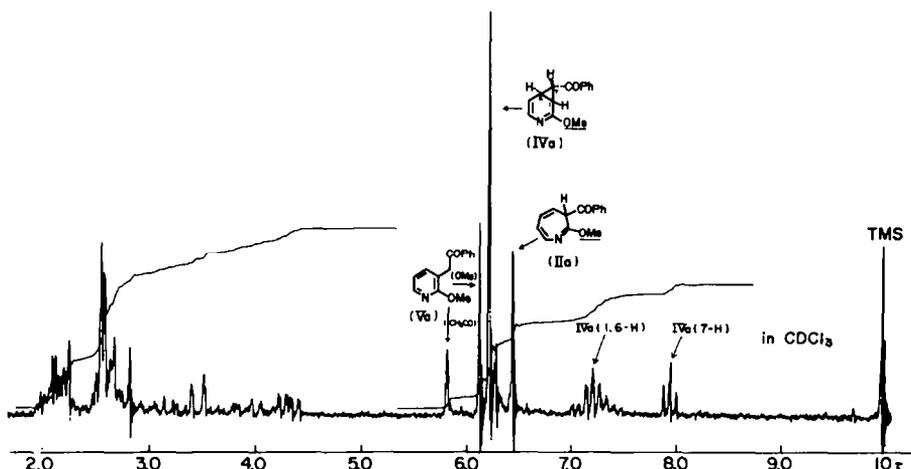
FIG. 1 NMR spectrum of Photoproduct mixture (IIa, IVa and Va).
